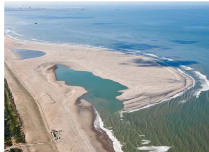
Sand Motor Project illustrating strategic sediment placement in the Netherlands.
